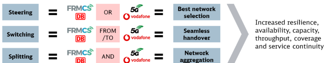
Figure 5.14: Steering, switching and splitting between connections provided by FRMCS and public 5G network as used by 5G-RACOM project
