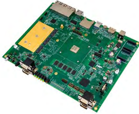
Figure 31: NXP LS1028A-RDB to implement UPF off-load.
